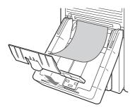
The output tray adapter prevents printouts from sticking out of the output tray.
